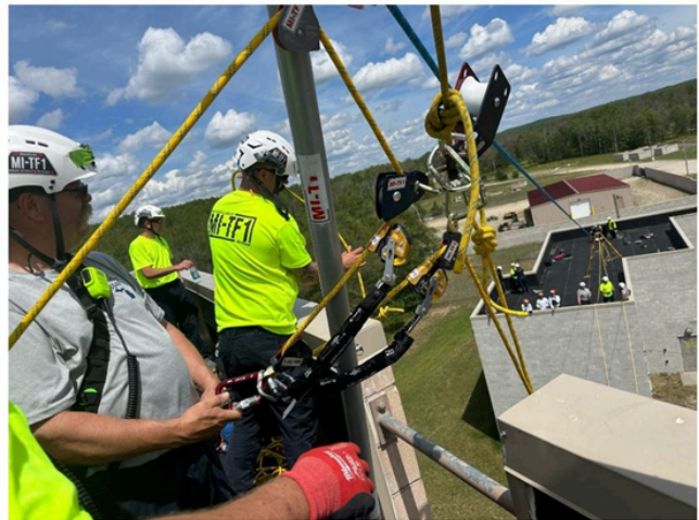
Here, team members build a highline rescue system between two buildings to transfer and lower a Taiwan rescuer to a trapped victim.
